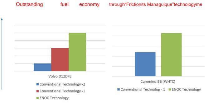
Advanced lubricant like ENOC Vulcan Energy 999X with 1% savings in fuel compared to conventional higher viscosity engine oils can yield huge fuel savings & reduction in CO2 emissions.
